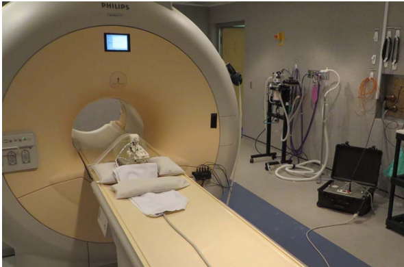
FIGURE 10. The master slave teleoperation system setup with a Philips Achieva 3 Tesla MRI scanner.
