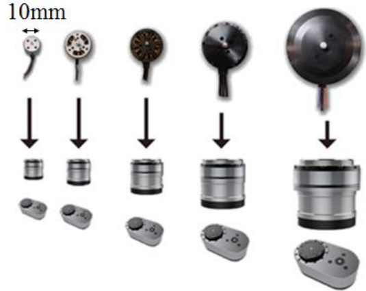
Fig 6. The size range of our custom-designed electric actuators are from 10mm to 100mm and have different output torque.
