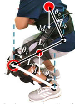
Fig. 6. The annotations for the mass of head, neck, thorax, abdomen, pelvis, arms, forearms, and hands ( M_b ), the mass of thigh ( M_t ), the length between the center of mass of M_b and the hip pivot ( L_b ), the length of thigh between the hip pivot and knee pivot ( L_t ), the length between the center of mass of M_t and the knee pivot ( L_{tc} ), the trunk angle ( \theta_b ), the thigh angle ( \theta_t ), and the shank angle ( \theta_s ).
